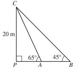
$$\begin{aligned} \tan 65^\circ &= \frac{20}{PA} \\ PA &= \frac{20}{\tan 65^\circ} = 9.326 \text{ m} \end{aligned}$$
